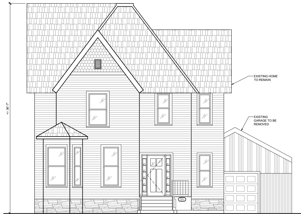
1 EXISTING FRONT ELEVATION - NORTHEAST SCALE: 1/4" = 1'-0"
