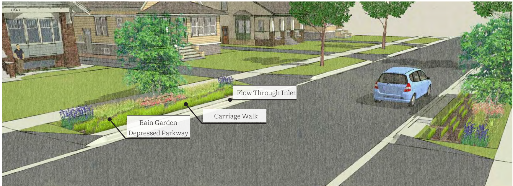
Figure 7.4. Stormwater Concept 1: Parkway Rain Garden
