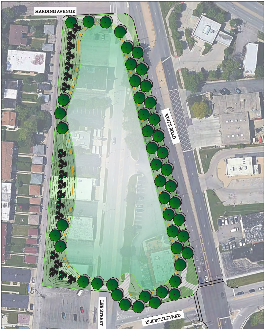
Figure 8.2. Stormwater Concept 4: Lee Street Stormwater Basin
