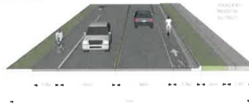
C12 Side Path-Arterial (no Median)
